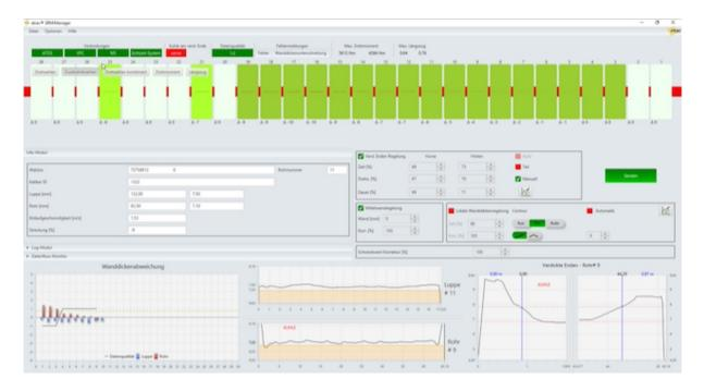
Setting data are always calculated and made available according to the current technological status for an upcoming new batch of rolling, immediately before rolling begins.
